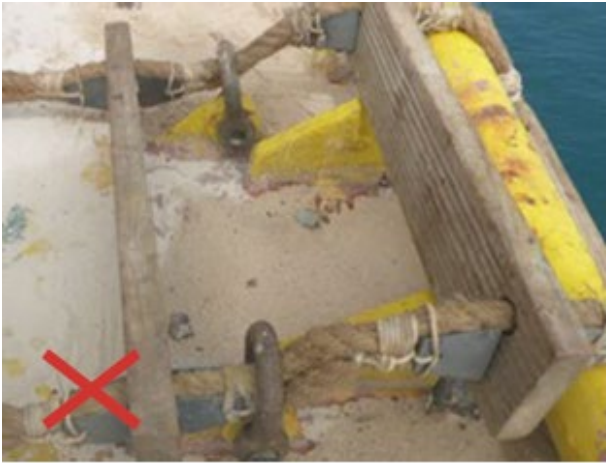
Secured using shackles, risk of damage to the chocks
