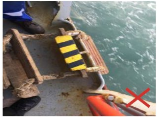
Secured using deck tongue, weight on the step
