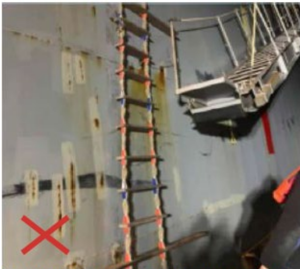
Distance of combination ladder from water line less than 5 metres
