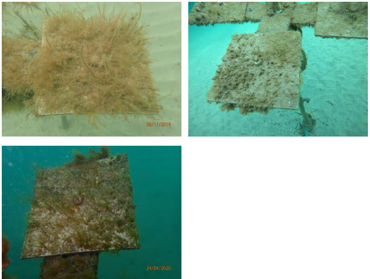
Figure 10: Settlement plates at site HRD at the end of the July-November 2019 deployment (top left), November 2019 – February 2020 (top right) and February-April 2020 (bottom left).
