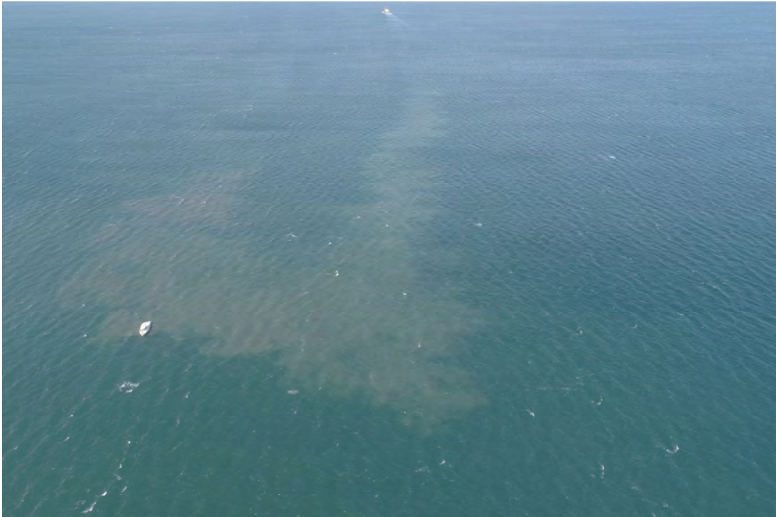
Figure 19: Dredge plume with the MAFRL sampling vessel in the foreground and the dredge moving off site in the background.
