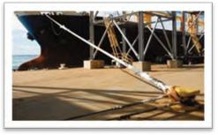
Shore Tension™ is a shore breast line that is passed from the shore to the vessel through the ship's centre leads fore and aft. This line is secured directly to the vessels' bollards. The tension on the line is controlled from the shore by way of hydraulic rams.
